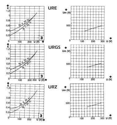
$<sup>^{\</sup>star}$  The mean curves show the variation of the total clearing time (I²t\_t) and the total clearing duration t\_t as a function of operating voltage U
